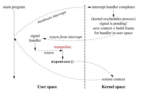
The kernel uses the signal trampoline to arrange that control is bounced back to kernel after execution of signal handler
